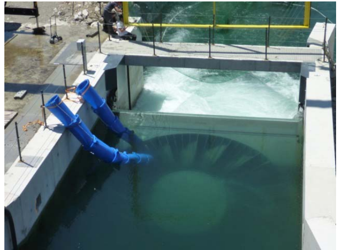
Injection tubes installed at mid-blade and at the runner periphery
