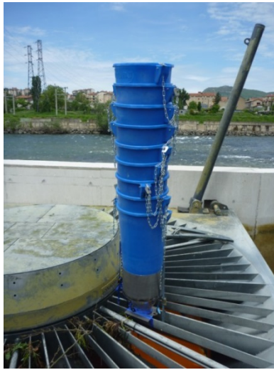
Stacked components of the injection tube
