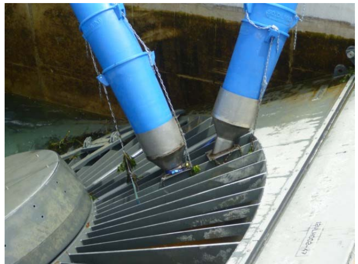
Injection tubes exit between the trash-rack bars - at mid-blade and at the runner periphery
