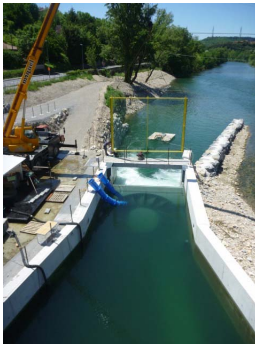
View of the VLH, with injection tubes and the frame of the recovery net.
