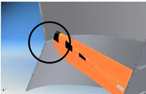
Figure 5. Discharge ring of the Troussy VLH and possible severing area at the blade tip
