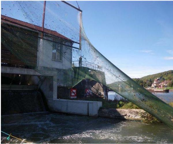
Image 11. View of the pocket formed where the mesh is the largest before entering the "sock" formed by the 2 finer meshes
