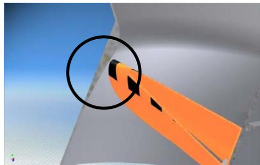
Figure 6. Spherical discharge ring at the blade tip of the new VLHs enabling to decrease the possible severing space
