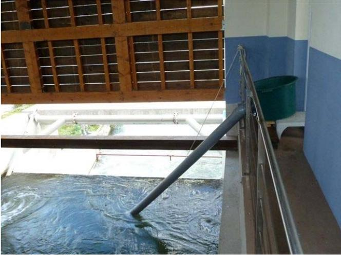
Image 3. Water tank connected to the PVC tube enabling to inject eels directly at the turbine guide vane level
