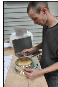
Dimensional check and tightness test on a bulb of one of the two DN 4000s of the Fraisans project
