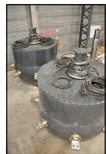
2 DN 4000 bulbs of the Fraisans project finished and under pressure test
