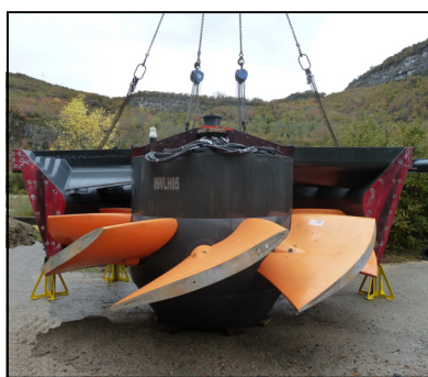
Turbina VLH DN 5000 w Yenne
