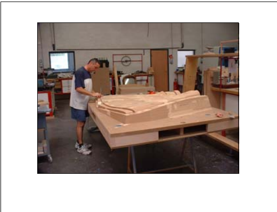
Wood and resin mould for the blade casting
